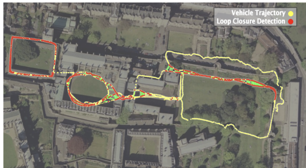
Figure 7: Appearance-based matching results for the New College dataset overlaid on an aerial photograph. The robot traverses a complex trajectory of 1.9km with multiple loop closures. 2,146 images were collected. Positions (from hand-corrected GPS) at which the robot collected an image are marked with a yellow dot. Two images that were assigned a probability p \geq 0.99 of having come from the same location (on the basis of appearance alone) are marked in red and joined with a line. There are no incorrect matches that meet this probability threshold. This result is best viewed as a video (Extension 1).
