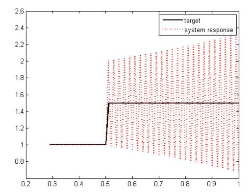
18)When a proportional controller tries to follow the step function (y=1: x<0.5; y=1.5: x>0.5) describe the possible causes for the response shown here:
