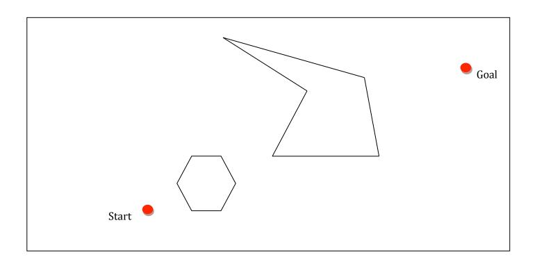
62) Draw the trajectory for the Bug2 path planning algorithm, starting position the robot goal the star. Consider a left turning robot.
