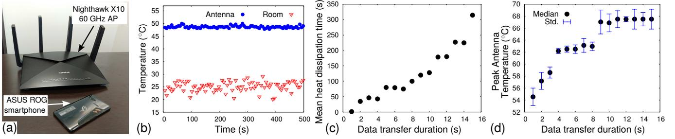
Figure 2: (a) Millimeter-wave access point (AP) and smartphone. (b) The temperature of the room and the millimeter-wave antenna at idle state. Effect of data transfer duration on: (c) Mean heat dissipation time; and (d) Peak antenna temperature.
