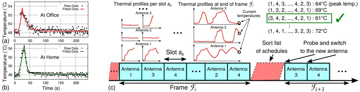
Figure 7: Data transfer for 10 s., and then, heat dissipation: (a) At office; and (b) At home. (c) *Aquilo* schedules antennas at the beginning of every frame  $\mathcal{F}_i$ ; then, probes and switches to a new antenna every slot  $s_k$ .
