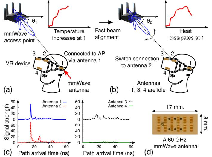
Figure 1: Core idea behind *Aquilo*: (a) VR device with 4 mmWave antennas connected to the access point (AP) via antenna 1; data transfer increases its temperature; (b) Scheduler switches to relatively cooler antenna 2 with the best link to the AP; (c) Signal strength of the best beam from the 4 antennas; (d) Dimensions of a 60 GHz mmWave antenna [8].
