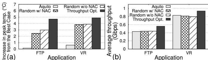
Figure 12: Performance in field trial applications: (a) System's peak temperature; (b) Application's throughput.
