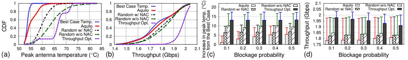
Figure 9: *Empirical CDF results from different schemes across various static conditions: (a) Peak antenna temperature; and (b) System’s throughput. Effect of increasing environmental blockage on the performance: (c) Increase in peak antenna temperatures from the best case; and (d) System’s throughput. The error bar shows 90<sup>th</sup> percentile value.*
