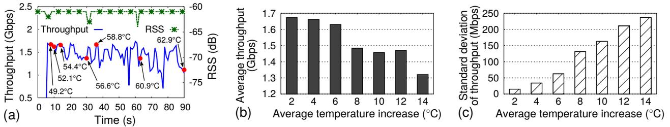
Figure 4: Link performance is affected by higher antenna temperature: (a) Link RSS is stable, but throughput fluctuates over time; every time index is marked for  $2^{\circ}\text{C}$  temperature increase; For every  $2^{\circ}\text{C}$  increase, we see changes in (b) Average throughput; and (c) Standard deviation of throughput.
