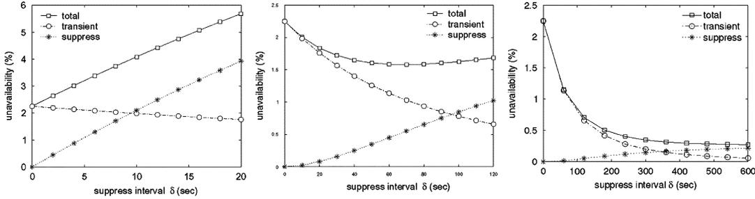
Fig. 8. Network unavailability. (a) OSPF. (b) FIR-1. (c) FIR-2.
