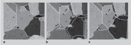
Figure 3. Segmentation of a (cropped) Ni-based alloy image by optimal labeling. (a) Segmented grain boundaries in a template slice. (b) Grain boundaries in (a) copied to a new slice. (c) Segmented grain boundaries in this new slice after optimal labeling.
