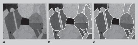
Figure 2. Segmentations on a (a) (cropped) Ni-based alloy image using (b) normalized cut and (c) ratio cut.
