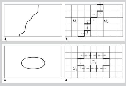
Figure 1. Image segmentation and graph cuts. (a) An image segmented by an open boundary. (b) The graph model for (a) and the graph cut for its segmentation boundary. (c) An image segmented by a closed boundary. (d) The graph model for (c) and the graph cut for its segmentation boundary.
