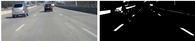
Fig. 5. (Left) Road with multiple lanes. (Right) Extracted lane markings that help identify the lane positions of the ego-vehicle and the detected vehicles.
