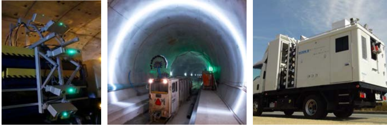
Figure 3. Three representative tunnel inspecting systems: Tunnelings, tCrack and MIMM-R.
