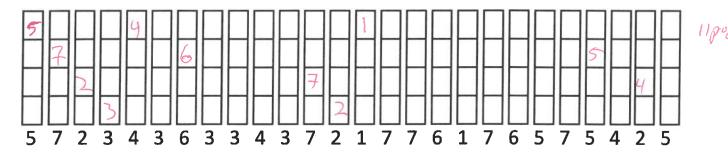
b. Construct the page replacement table for LRU algorithm and record how many page faults. Fill in the page table after each reference.
