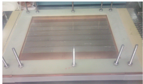
Figure 6. An HDPE rolling pin was used to flatten the lithium onto the bottom and top (not shown) copper plates before the wire frame is put in place.
