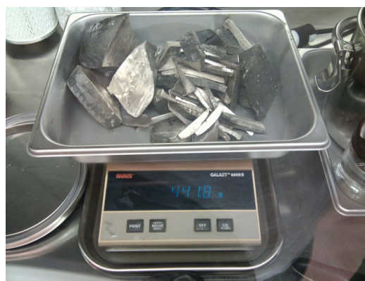
Figure 2. 440 g of lithium “chunks” purchased from Y-12/Oak Ridge National Laboratory, which were received in mineral oil and had a thin (100 micron) blackened layer. The chunks were cut open for rolling experiments. The open surfaces reveal the silvery-white untarnished lithium material.
