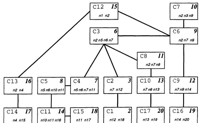
FIG. 12. Junction tree of cliques derived from perfect ordering of the CHLD nodes. The members of each clique are shown, the highest label among the members is shown in the top right-hand corner, while the corresponding ordering of the cliques is shown in the top left-hand corner.
