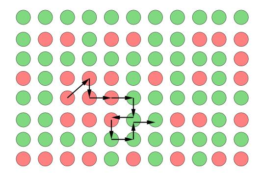
Reachable in one step: instantiations that differ from current one by value assignment to at most one variable (assume randomized choice of variable  $V_k$ ).
