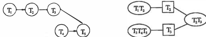
Figure 4.1 The Bayesian network M_{\min} and a corresponding cluster tree. Separators are in square boxes.
