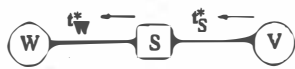
Figure 4.2 W absorbs from V . t_S^* = \sum_{V \setminus S} t_V ; t_W^* = t_W \cdot \frac{t_S^*}{t_S} .
