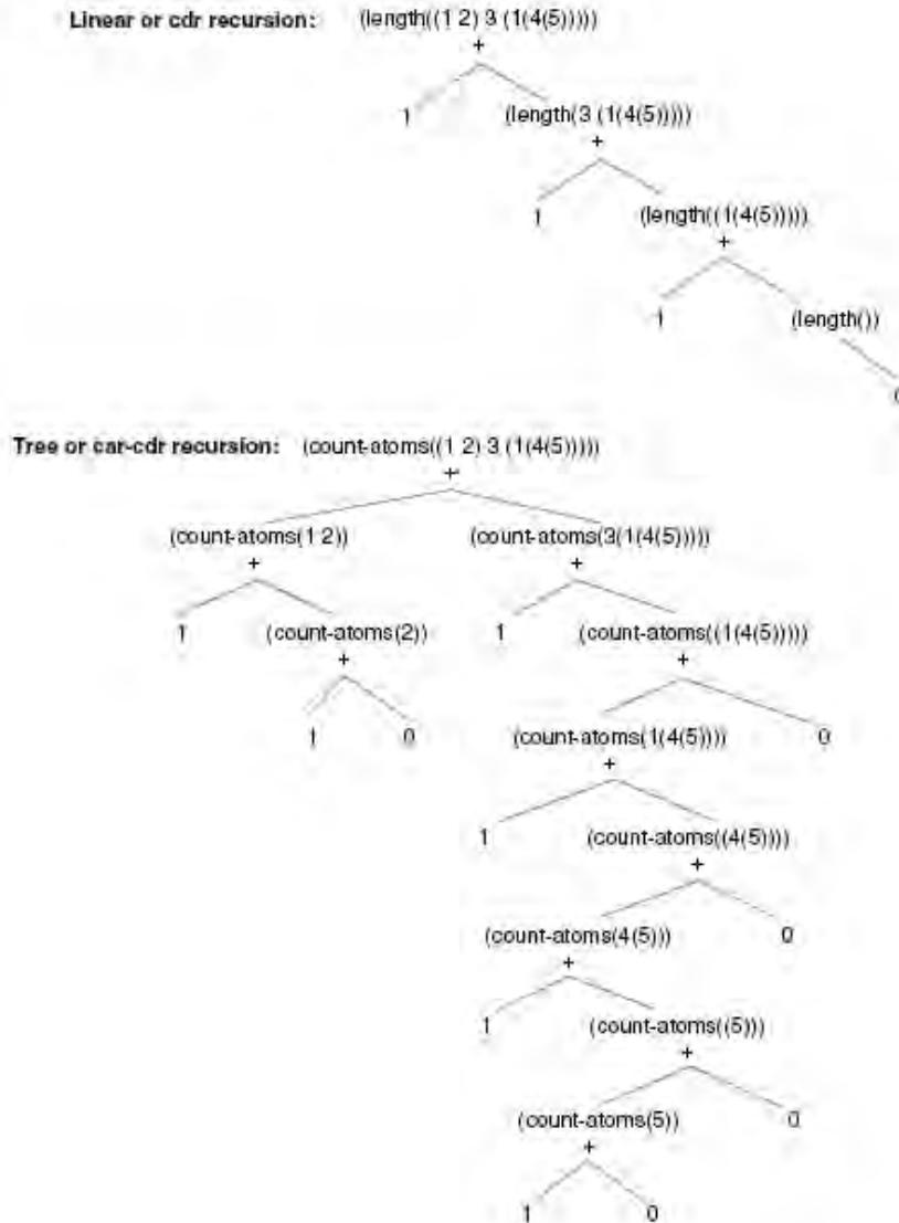
**Figure 12.2. Tree representations of linear and tree-recursive functions.**
