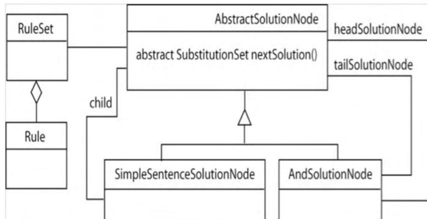
**Figure 24.9.** The class structure for implementing continuations.
