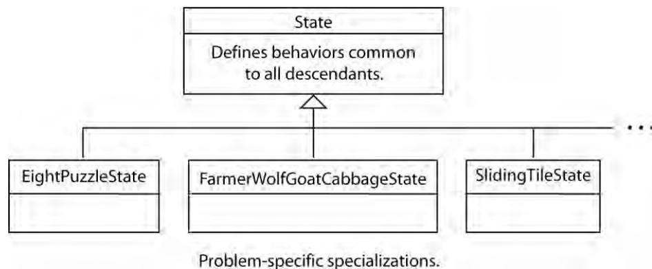
**Figure 22.3. State representation for search containing problem-specific specifications.**
