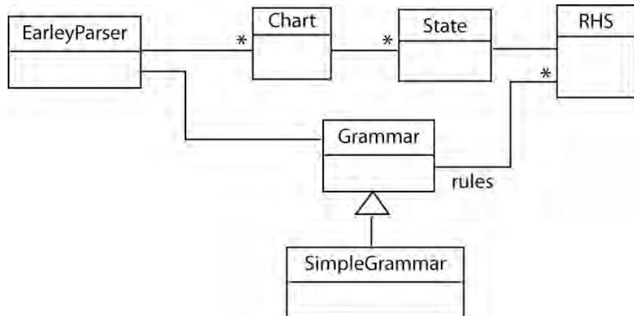
Figure 30.1 The design hierarchy for the EarleyParser class.
