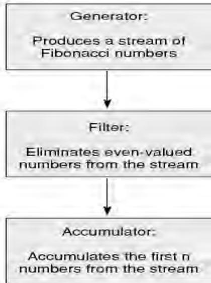
**Figure 17.1. A stream implementation that finds the first  $n$  odd Fibonacci numbers.**
