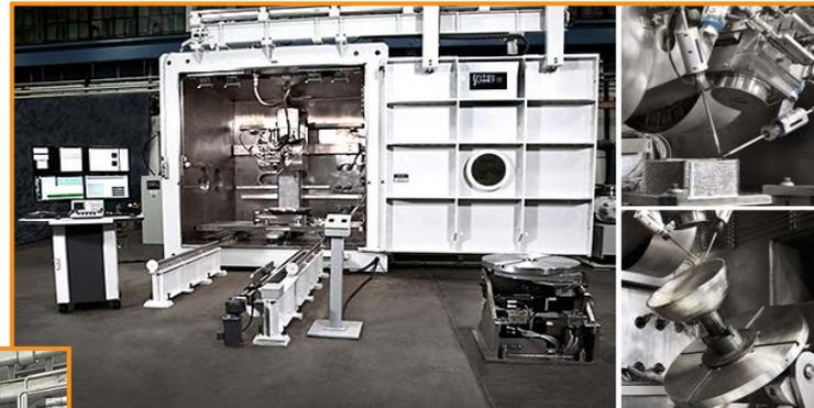
E-beam Additive Manufacturing System
