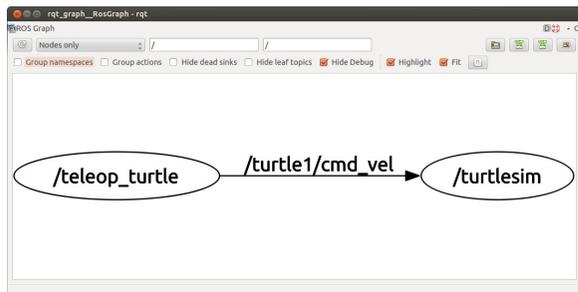
Figure 2.2: The `rqt_graph` interface, showing the graph for the `turtlesim` example. Debug nodes, including `roscout`, are omitted by default.
