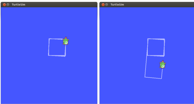
Figure 9.3: [left] A turtlesim turtle responding to movement commands from draw_square. Those movement commands are also recorded by rosbag. [right] By replaying the bag, we can send the same sequence of messages to the turtle.
