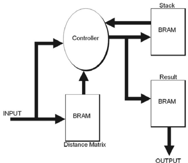
Fig. 5. Block diagram of tree search processing element.
