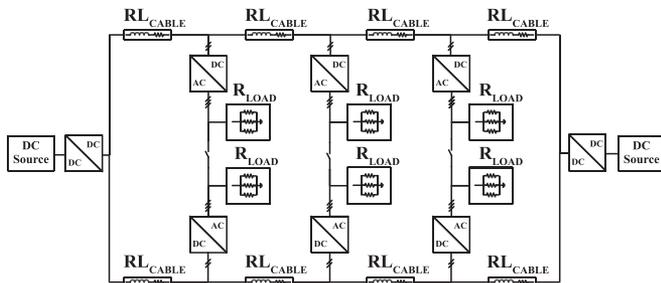
Fig. 10. Dual bus shipboard power system.
