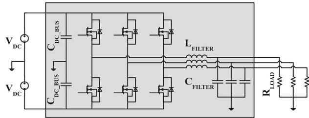
Fig. 8. Three phase DC/AC converter.
