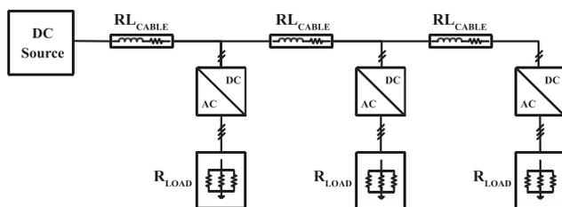
Fig. 9. Single bus shipboard power system.
