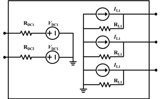
Fig. 5. DC/AC converter system solver structure.
