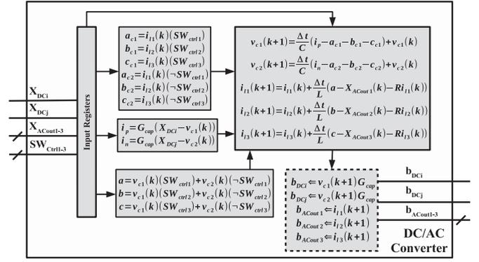
Fig. 3. Example of DC/AC converter component entities.
