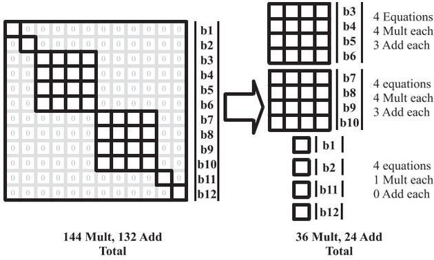
Fig. 4. Separation of subsystems.
