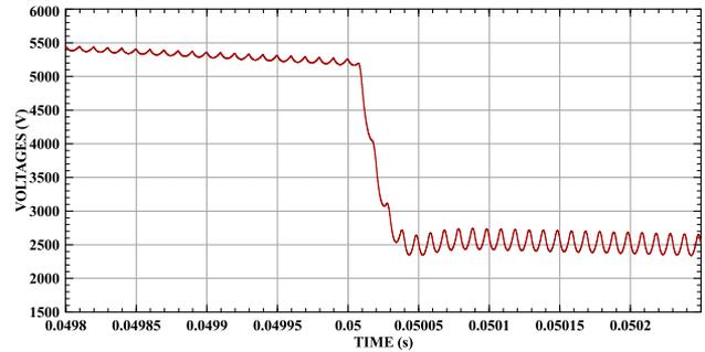
Fig. 14. Single-bus power system analog output, phase 1 zoom.
