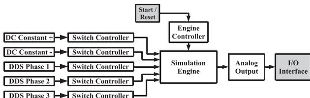
Fig. 11. Top level design for simulation platform.
