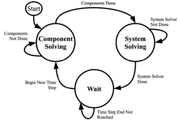
Fig. 7. Finite state machine for multi-cycle simulation engine.
