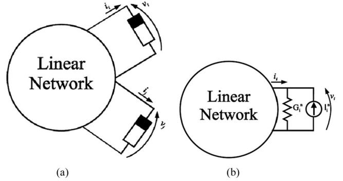
Fig. 1. Linear networks with nonlinear components. (a) With two nonlinear components. (b) With one current-type nonlinear component.
