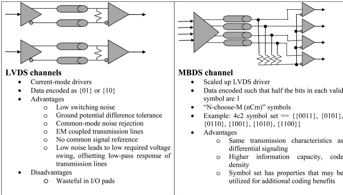
Fig. 1. Side-by-side comparison of LVDS and MBDS channels.
