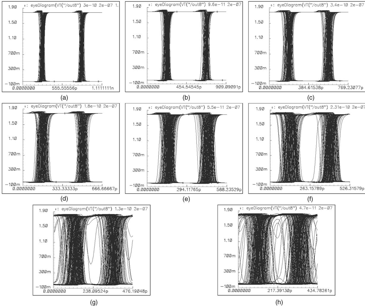
Fig. 9. Eye diagrams of one receiver output as symbol transmission rate is scaled along the following scale: (a) 1.8 GHz, (b) 2.2 GHz, (c) 2.6 GHz, (d) 3.0 GHz, (e) 3.4 GHz, (f) 3.8 GHz, (g) 4.2 GHz, and (h) 4.6 GHz.
