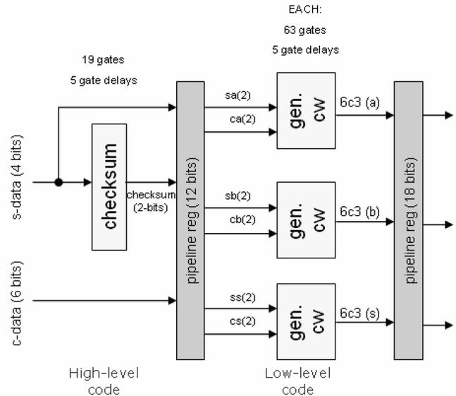
Fig. 3. Example encoder architecture.
