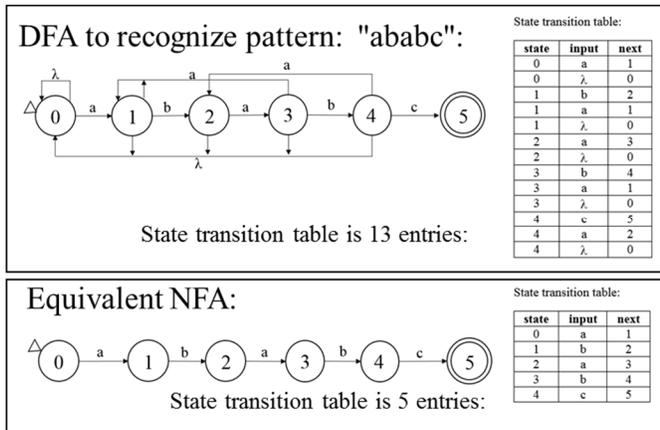
Fig. 1. DFA vs. NFA and conversion of NFA with edge labels to state labels.
