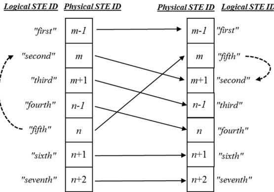
Fig. 3. Remapping physical STEs. Edge between logical STE “fifth” and “second” is reassigned from physical STEs  $n$  and  $m$ , where  $n > m$ , to  $m$  and  $m+1$  (after an operation “move STE  $n$  to  $m$ ”). In this case, a movement from a higher-numbered STE to a lower-numbered STE causes all other STEs assignments between the two values to shift up, requiring an update to all other edges involving these physical STEs.
