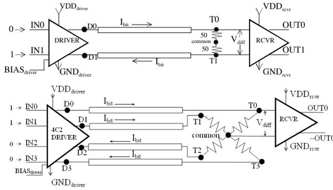
Figure 5. Electrical model of 2C1 link (top) and 4C2 link (bottom)
