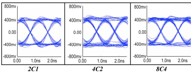
Figure 3. Comparative eye diagrams from simulations of 2C1, 4C2, and 8C4 MBDS links
