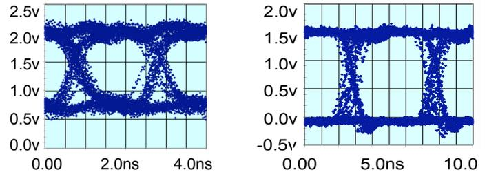
Figure 4. 500Mbps eye diagram: test link with custom receiver (left), 200Mbps eye diagram: test link with commercial LVDS receiver (right).
