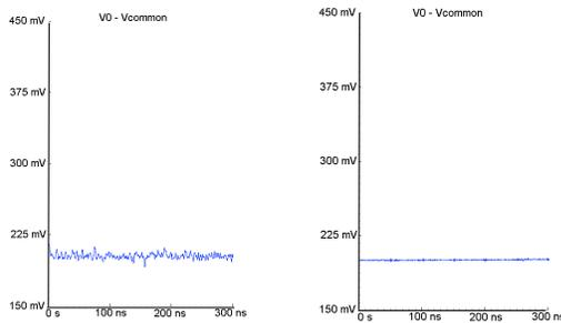
Figure 7. Simulation data for common mode noise rejection. Output signal measured between nodes  $V_{T0}$  and  $V_{COMMON}$  in Figure 5 for (LEFT) 50mV AWGN added to bias input, and (RIGHT) using four 200mV coherent sources at nodes D1, D2, D3, and D4.
