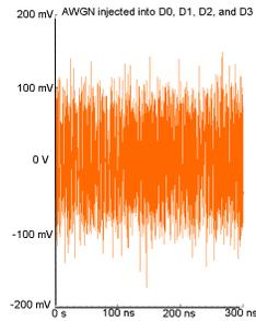
Figure 6. Additive white Gaussian noise (AWGN) signal used in common mode noise rejection simulations.
