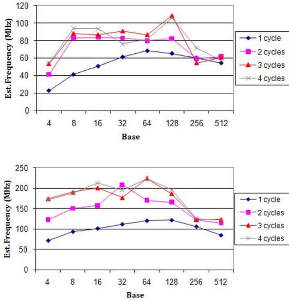
Fig. 2. Synthesis results for Virtex 2 Pro 100 (top) and Virtex-5 LX 330T (bottom), as operating frequency versus base value.
