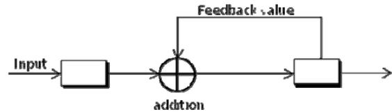
Fig. 1. Serially-delivered accumulator.
