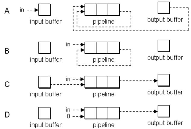
Fig. 5. Configuration states for the reduction circuit.
