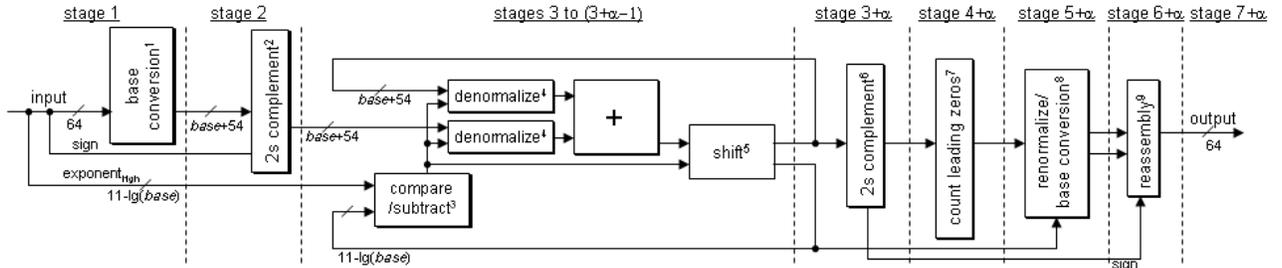
Fig. 3. Top-level design of accumulator architecture. Alpha represents the pipeline latency of addition datapath.
