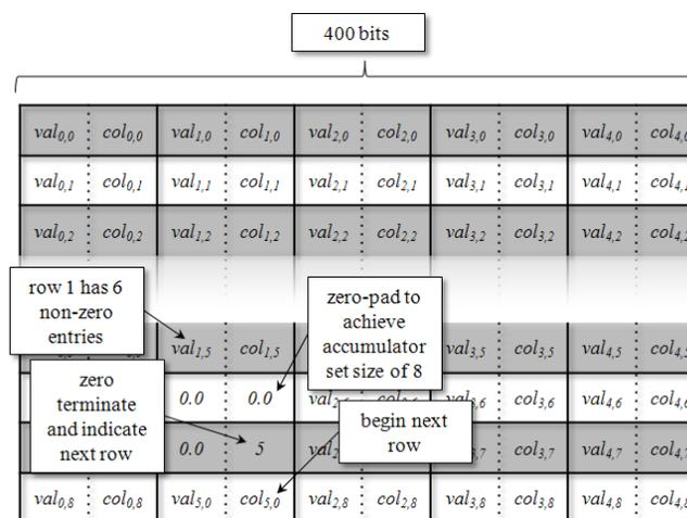
**Fig. 7. Matrix data scheduling technique.** In this case, 400-bit “packets,” that are read each cycle, are composed of five “slots”—one for each accumulator.
