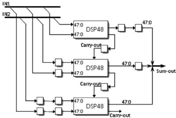
Fig. 4. Pipelined, cascaded DSP48 blocks forming a wide adder.
