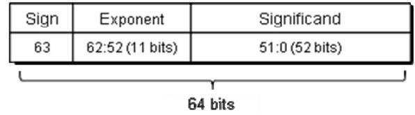
Fig. 2. IEEE 754 Double Precision Floating Point Format
