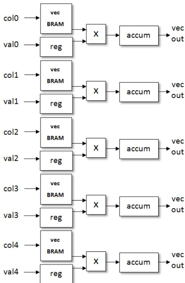
**Fig. 6. SpMV Architecture.** The FPGA can read five matrix values and their corresponding column values per cycle. The FPGA associates a copy of the input vector, a multiplier, and an accumulator with each.
