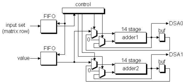
Fig. 2. DSA Reduction Circuit Design from [4].
