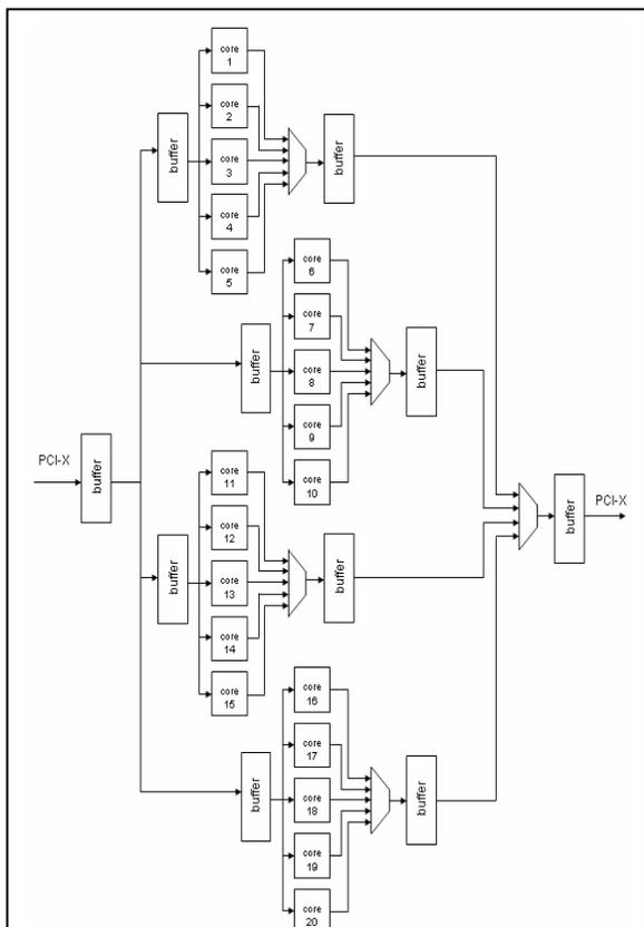
Figure 9. Simplified block diagram for the top-level FPGA implementation of a 20-core design. Due to the high clock speed requirement for the PCI-X interface (an independent clock domain from the slower core clock), the fan-outs and fan-ins are pipelined with degree 4 and 5. Dual-ported split clock BRAMs are used for the input and output data to cross clock domains.
