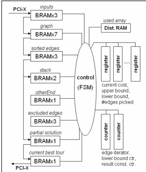
Figure 7. Simplified block diagram for the breakpoint median core. The core design is a large sequential logic circuit that establishes datapaths among several memory elements in each clock cycle. Static interconnects between memory elements are shown, while multiplexed interconnects among memory elements are established through the control unit (integrated within its output logic).
