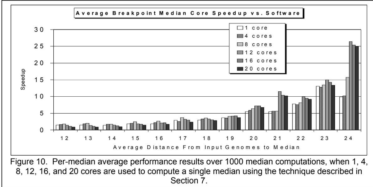
Figure 10. Per-median average performance results over 1000 median computations, when 1, 4, 8, 12, 16, and 20 cores are used to compute a single median using the technique described in Section 7.
