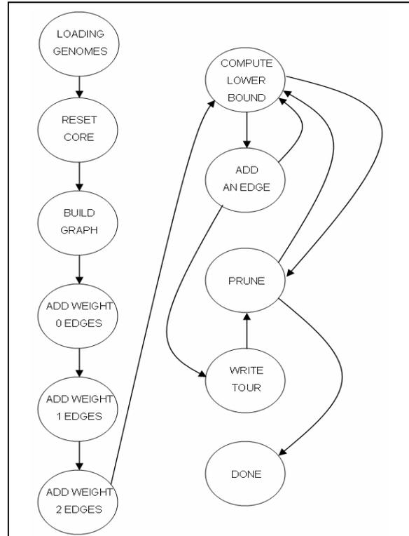
Figure 8. Finite state machine representation of median core controller.
