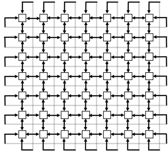
Fig. 3: Torus topology, 4 channels/node, worst case latency =  $\sqrt{n}/2$ .
