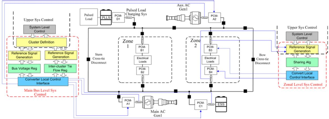
Fig. 1. Portion of a notional shipboard power system with communication among converters' control systems.
