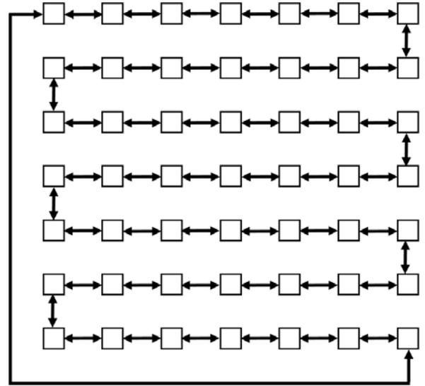
Fig. 2: Ring topology, 2 channels/node, worst case latency =  $n/2$ .
