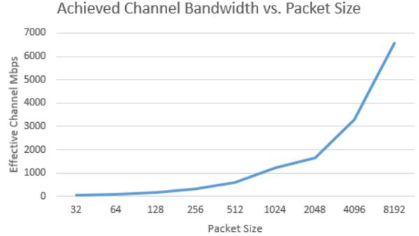
Fig. 8: Observed Aurora channel bandwidth versus packet size.
