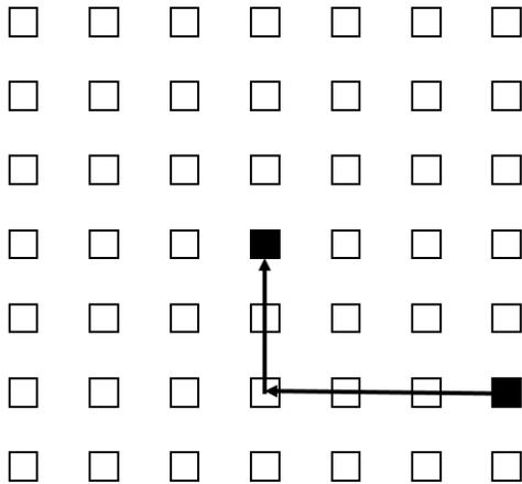
Fig. 4: X-Y Routing.
