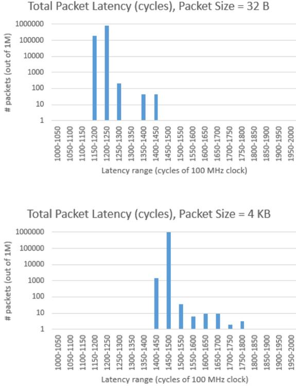
Fig. 7: Observed packet transmit latency for 32 byte packets (top) and 4 Kilobyte packets (bottom). These results include packet transmission time over the 10 Gbps link (~3 cycles for a 32 byte packet and ~328 cycles for a 4KB packet) and the platform overheads, such as those contributed by the on-chip interconnect, DMA engines, interrupt controller, and driver software. Note that the Y-axis is logarithmic.
