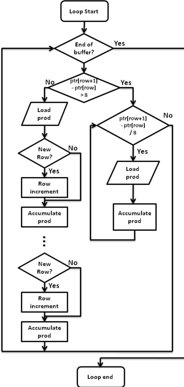
Fig. 2. Adaptive Accumulation Loop
