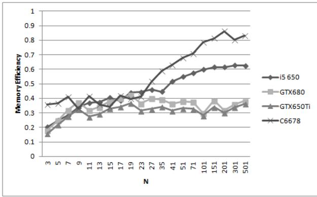
Fig. 7. Memory Efficiency on N-diagonal Matrices
