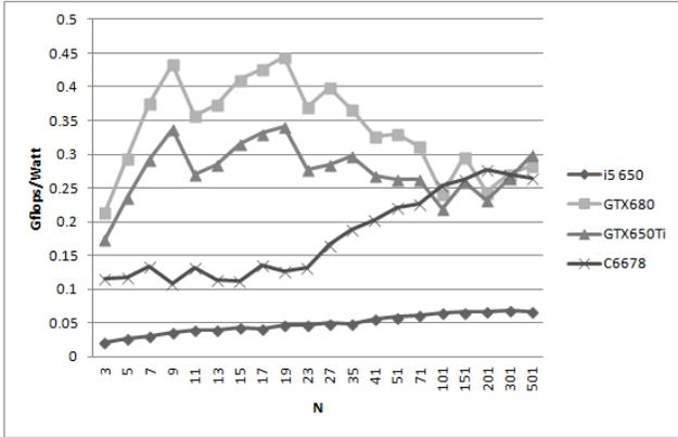
Fig. 4. SpMV Gflops/Watt on N-diagonal Matrices
