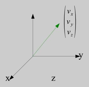
$$\begin{vmatrix} v_x \\ v_y \\ v_z \end{vmatrix} = \begin{vmatrix} r\sin(\theta)\cos(\phi) \\ r\sin(\theta)\sin(\phi) \\ r\cos(\theta) \end{vmatrix}$$
