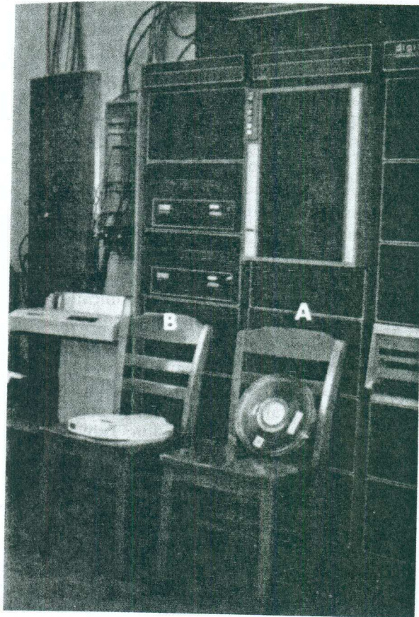
Figure 2.5a Mass storage devices used on PDP 11/55 minicomputer. A: Magnetic tape, B: Moving head disks.
