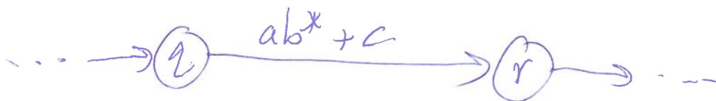
Can get directly from  $q$  to  $r$  by reading some string from the input that matches  $ab^* + c$ , i.e., a followed by 0 or more  $b$ 's or a single  $c$ .
