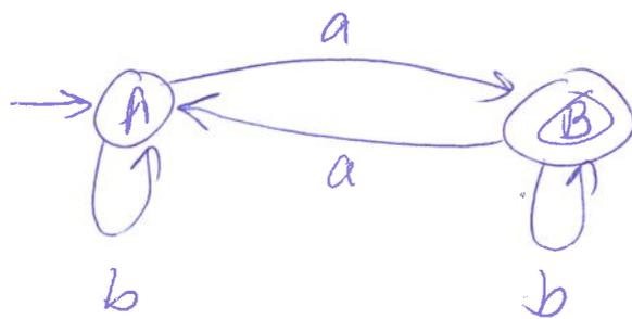
$L(N) = \{w \in \{a,b\}^* \mid w \text{ has an odd \# of } a\text{'s}\}$
