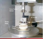
pin-on-disk module with 1000°C chamber
