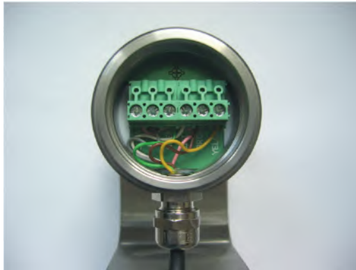
Fig. 11 View on terminal block with sensor cables
