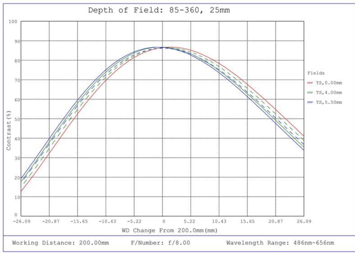
#85-360, 25mm, f/8 Ci Series Fixed Focal Length Lens, Depth of Field Plot, 200mm Working Distance, f8
