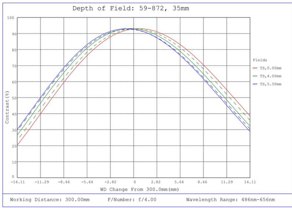
#59-872, 35mm C Series Fixed Focal Length Lens, Depth of Field Plot, 300mm Working Distance, f4
