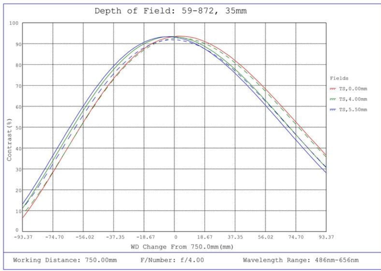
#59-872, 35mm C Series Fixed Focal Length Lens, Depth of Field Plot, 750mm Working Distance, f4
