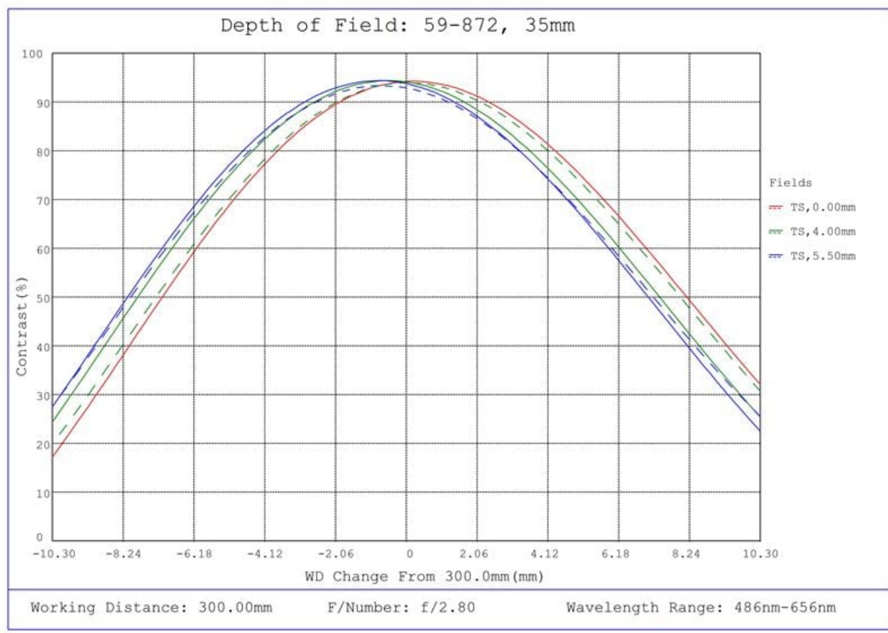
#59-872, 35mm C Series Fixed Focal Length Lens, Depth of Field Plot, 300mm Working Distance, f2.8
