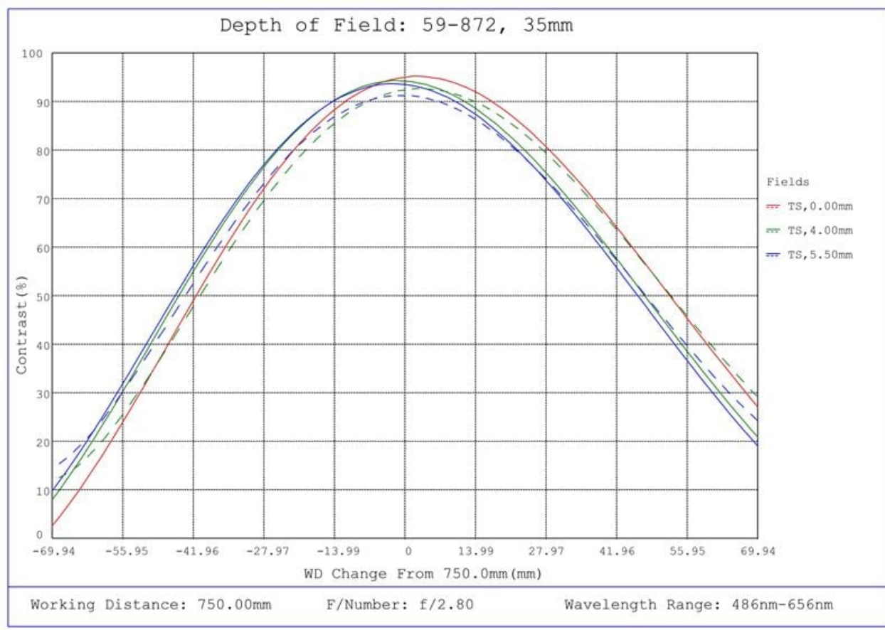
#59-872, 35mm C Series Fixed Focal Length Lens, Depth of Field Plot, 750mm Working Distance, f2.8
