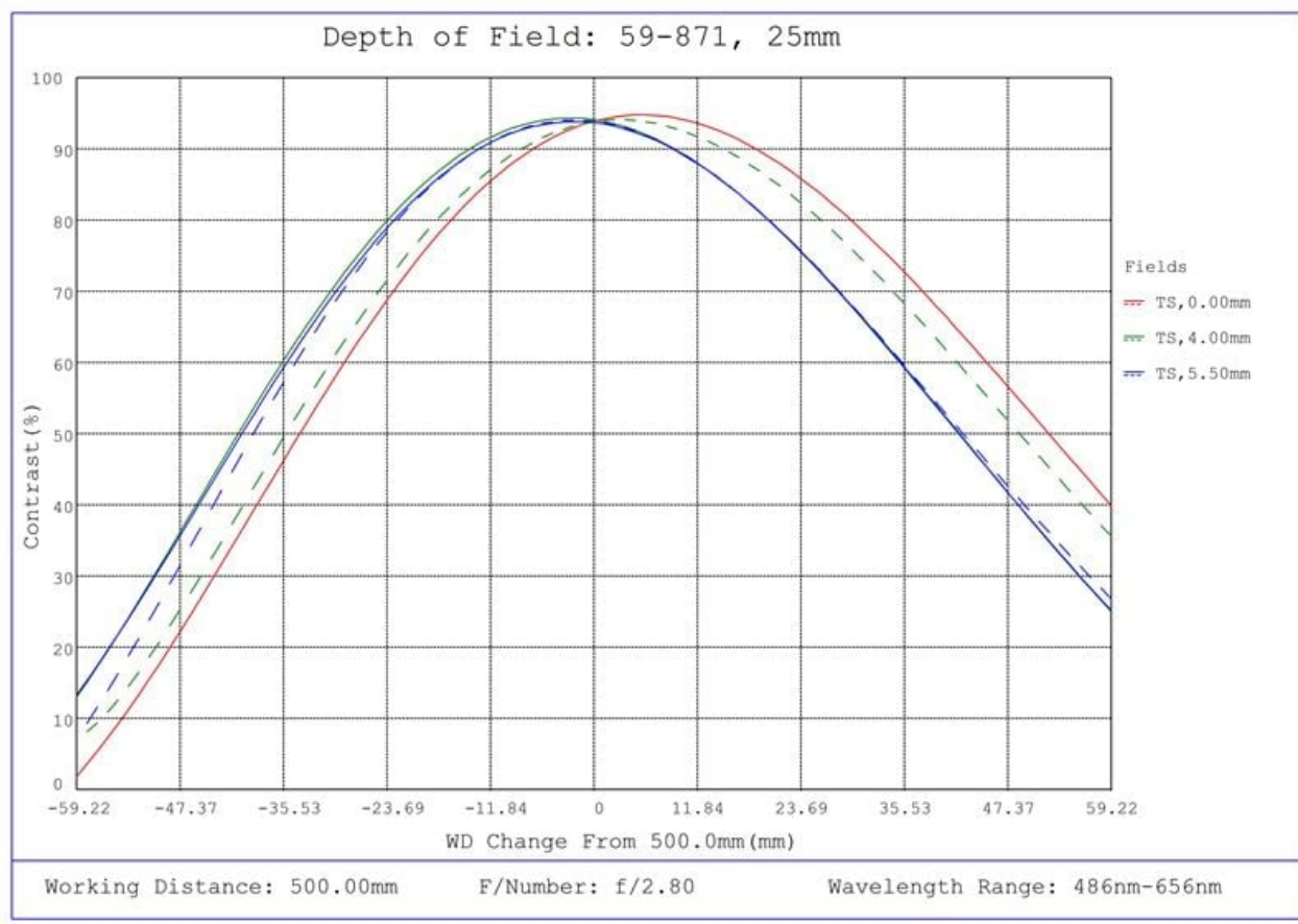
#59-871, 25mm C Series Fixed Focal Length Lens, Depth of Field Plot, 500mm Working Distance, f2.8
