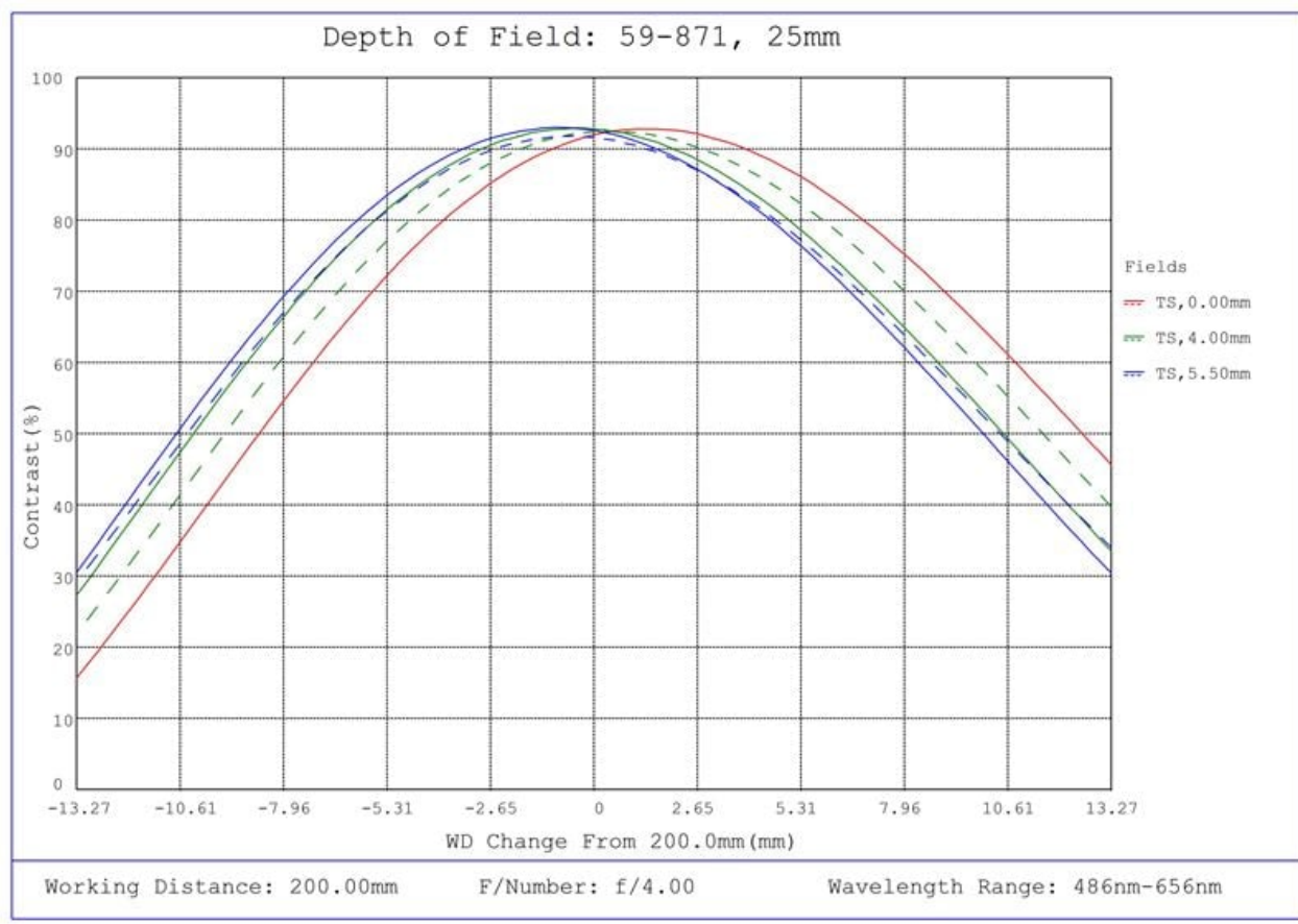
#59-871, 25mm C Series Fixed Focal Length Lens, Depth of Field Plot, 200mm Working Distance, f4
