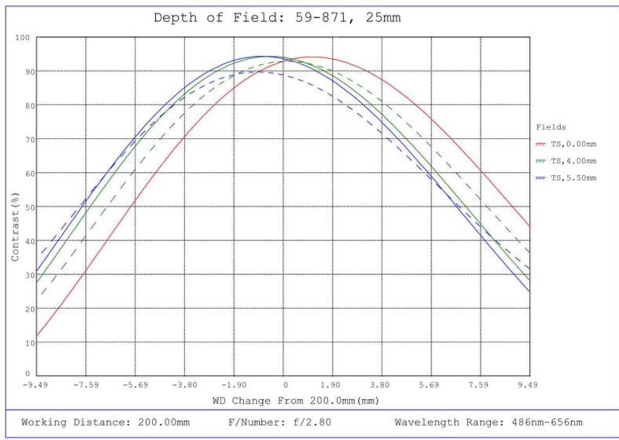
#59-871, 25mm C Series Fixed Focal Length Lens, Depth of Field Plot, 200mm Working Distance, f2.8
