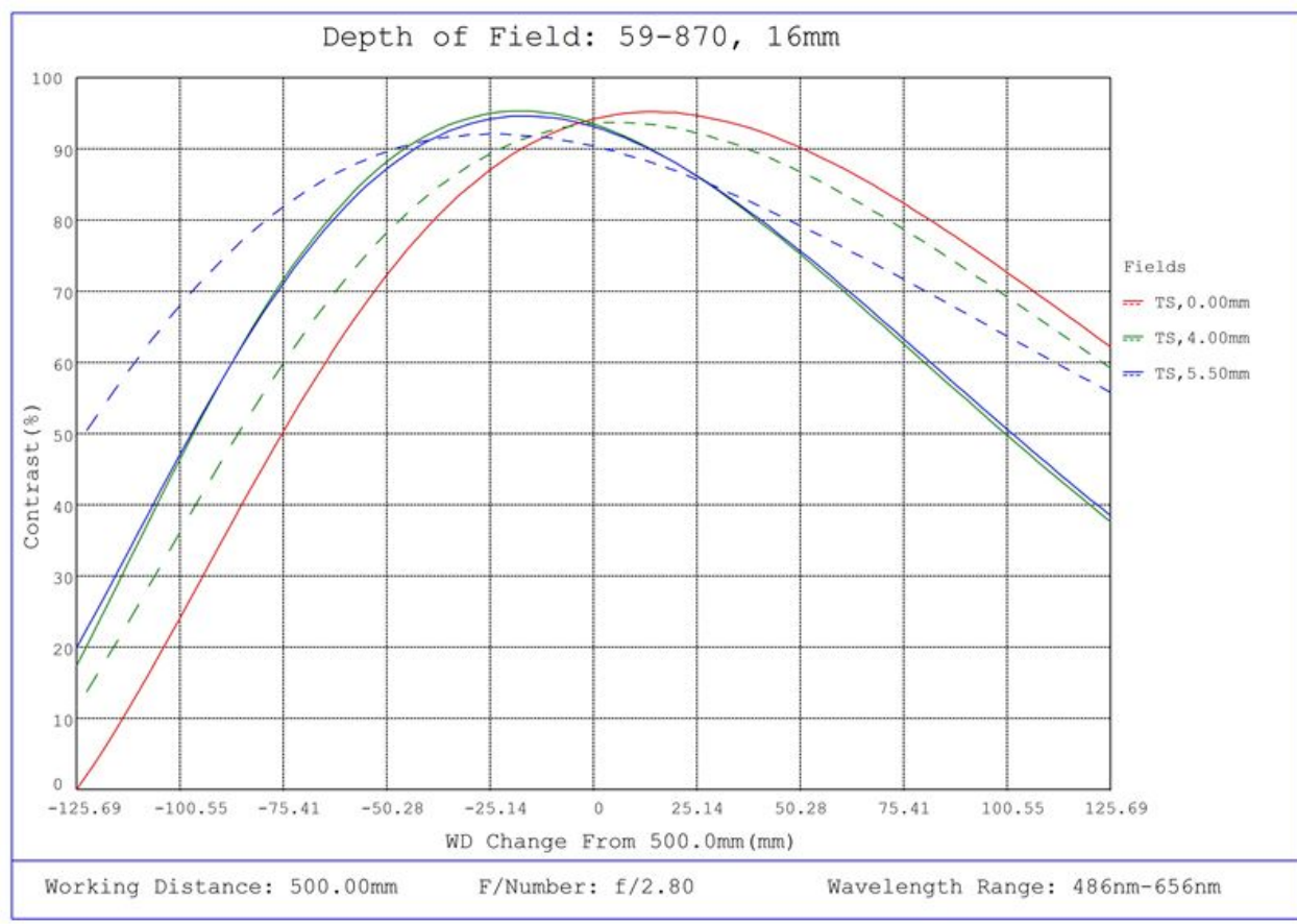
#59-870, 16mm C Series Fixed Focal Length Lens, Depth of Field Plot, 500mm Working Distance, f2.8
