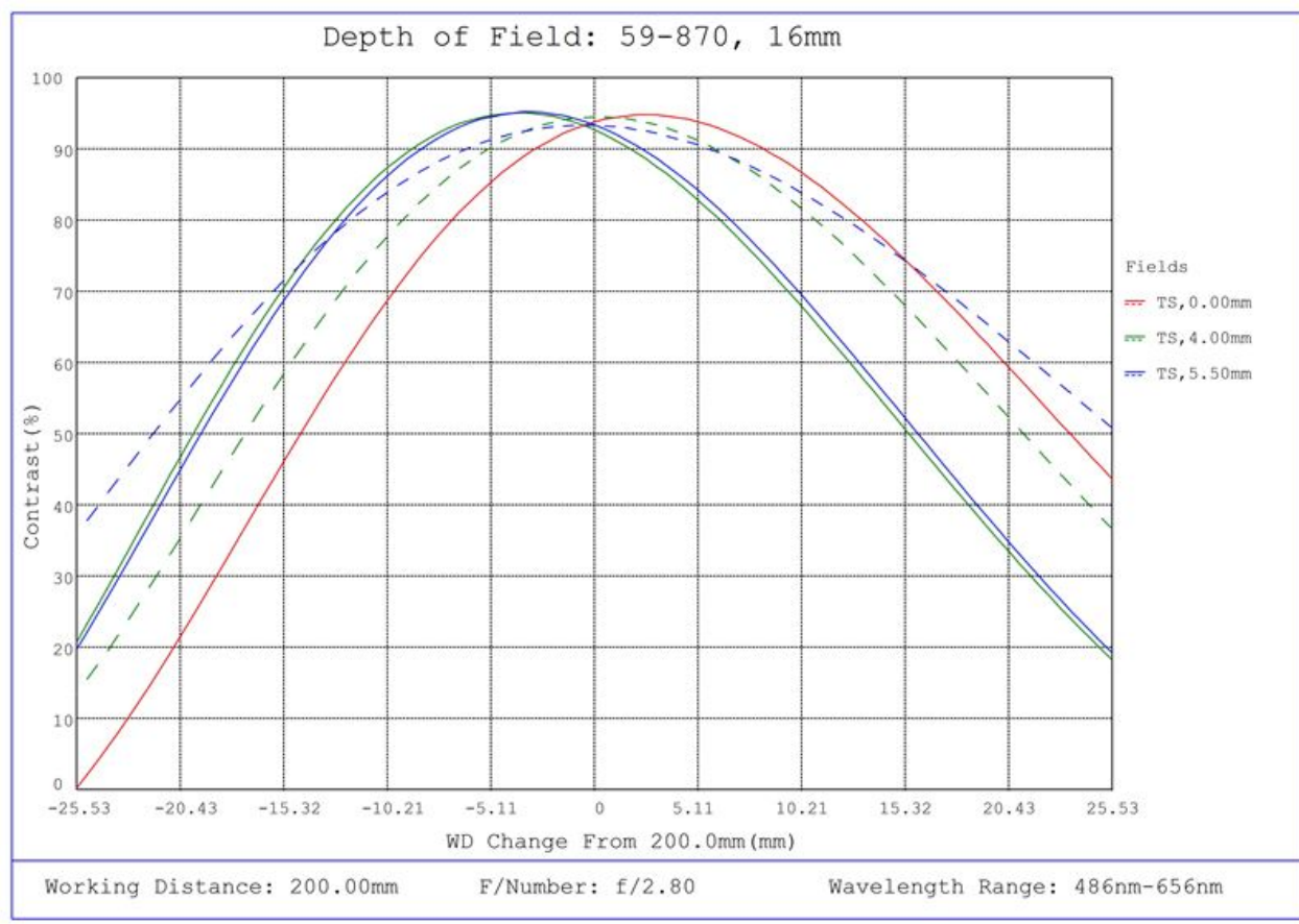
#59-870, 16mm C Series Fixed Focal Length Lens, Depth of Field Plot, 200mm Working Distance, f2.8
