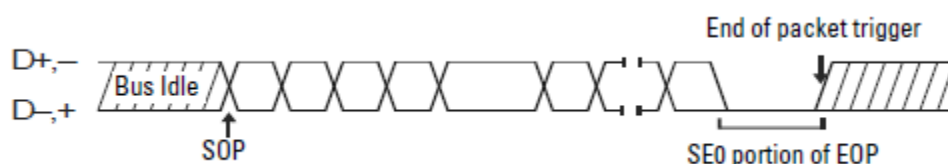
Figure 5-8 USB Data Transmission Protocol
