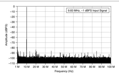
$<sup>^{16}</sup>$  Excludes harmonics. 10 MHz, -1 dBFS input signal. Measured from DC to 100 MHz.
