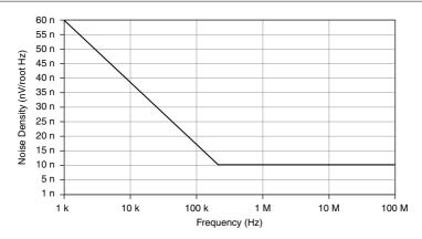
Figure 4. PXI-5124 Spectral Noise Density on 0.2 V Input Range, Full Bandwidth, 50 Ω Input Impedance, Nominal
