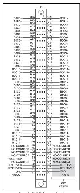
Figure 2. NI 2529 Connector Pinout
