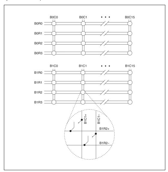
Figure 1. NI 2529 Power-On State
