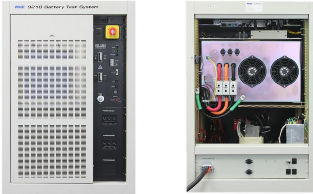
Figure 1 - 9210 System with 4904 Module (Safety screen removed to show isolation transformer)
