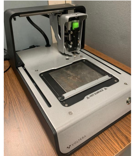
Figure 2. Voltera desktop printer with metal build plate.
