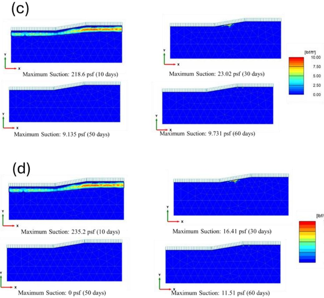
**Figure 7: Matrix Suction for 100 years and 500 years rainfall in McRaven Road (a) displacements for 100 years rainfall with 15 mins duration, (b) displacement for 100 year rainfall with 30 mins duration, (c) displacements for 500 years rainfall with 15 mins duration, (d) displacement for 500 year rainfall with 30 mins duration**
