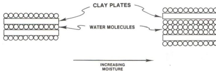
**Figure 2: Physical change in expansive clay due to moisture**
