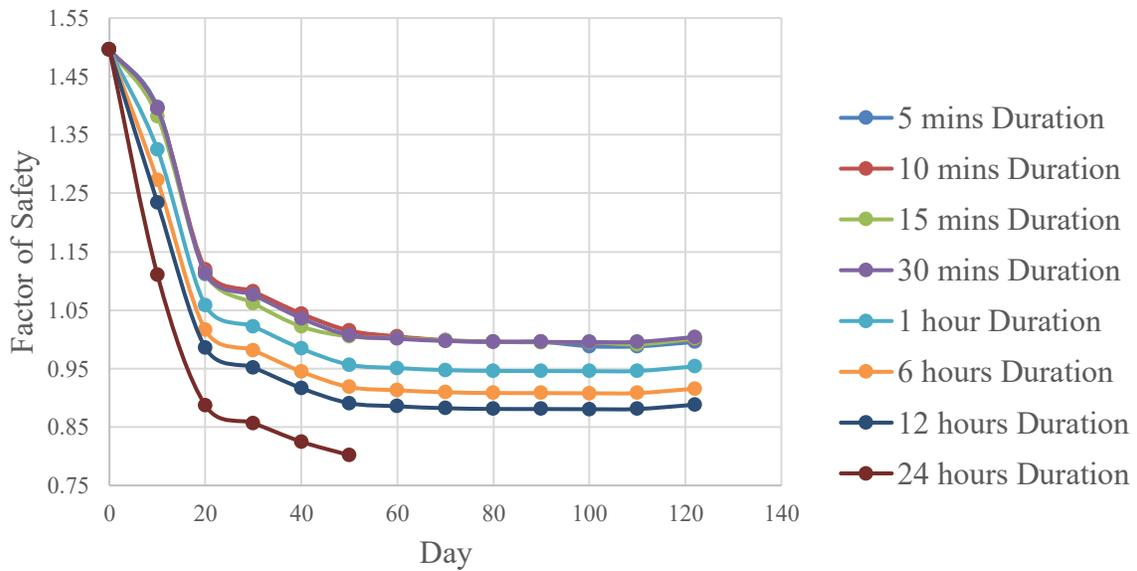
Figure 8: Change of FS with (a) 100-years and (b) 500-years rainfall return period at various duration
