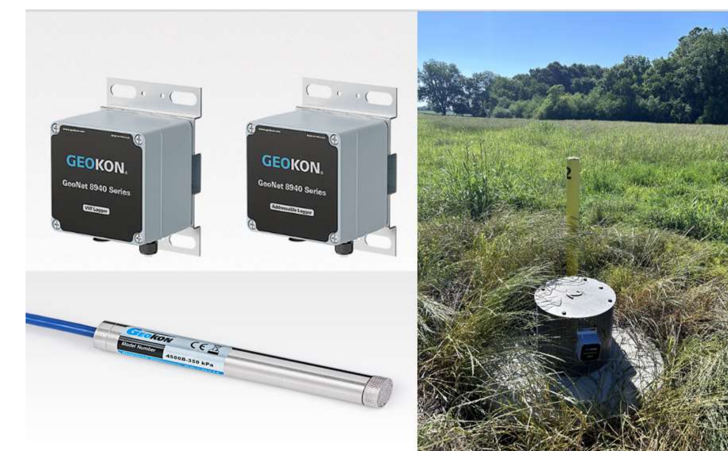
Figure 3. Geokon data logger and VW piezometer installation at Norfolk site 1.
