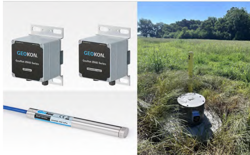
Figure 4. (a) Geokon 8940 series data logger (b) Geokon 4500B VW Piezometer sensor (c) Piezometer installation at Norfolk 1 site.
