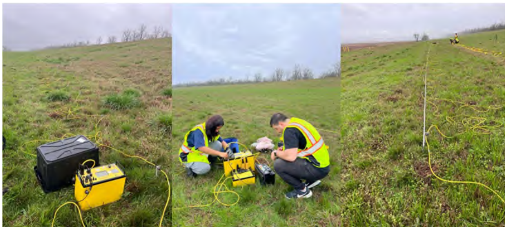
Figure 3. ERI test equipment and survey line placement.
