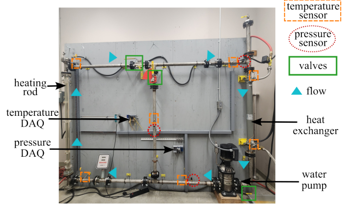
FIGURE 4: Physical primary loop thermal-hydraulic testbed used to emulate reactor heat generation and coolant circulation with instrumented sensors.
