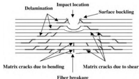
Damage propagation in a woven composite. [dfwptp.com](http://dfwptp.com)
