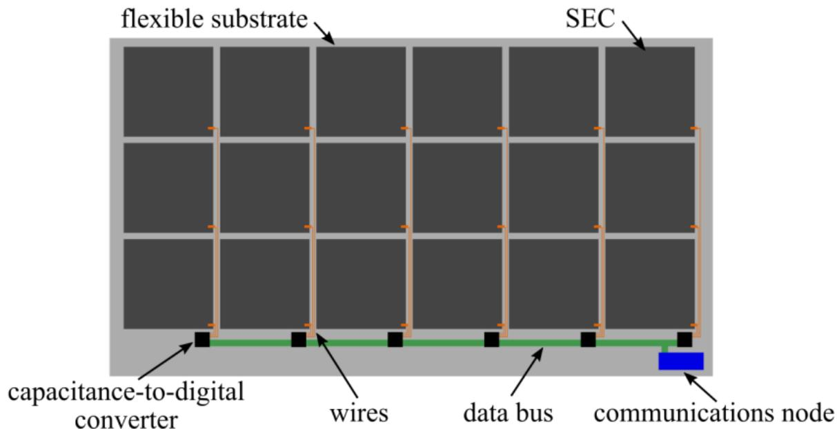
Yan et al., "Surrogate model for condition assessment of structures using a dense sensor network".
