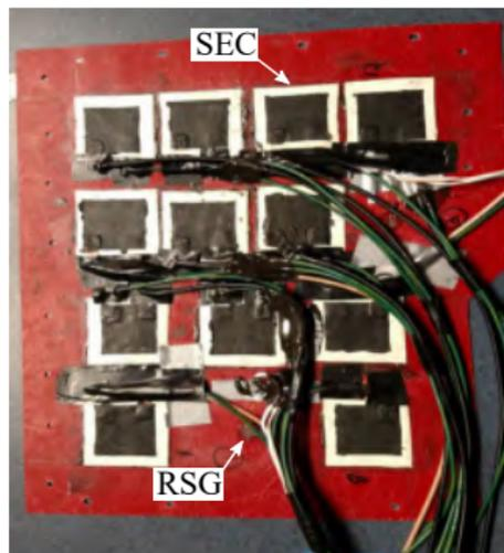
DSN installed inside model
