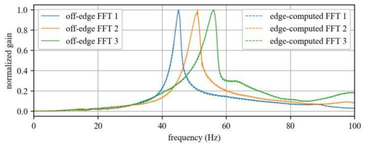
🔴 Mode 1 Frequency: 45.1 Hz 🛑 Mode 1 Frequency: 51.0 Hz 🌑 Mode 1 Frequency: 56.0 Hz
