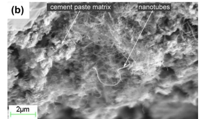
SEM image of cement paste with MWCNTs magnified 25,000 times.
