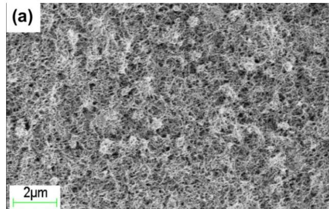
SEM image of MWCNTs-water solution magnified 50,000 times.
