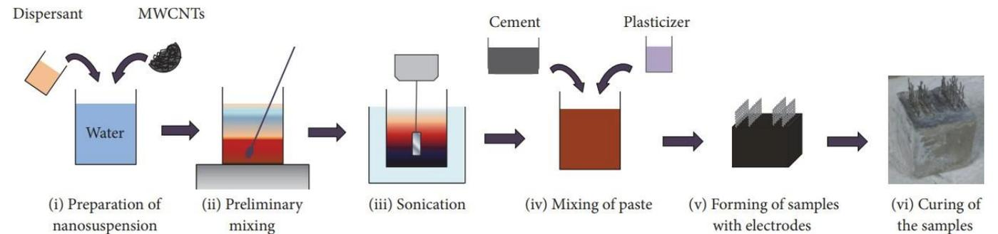
Preparation process of the cement paste samples with 1% of MWCNTs
