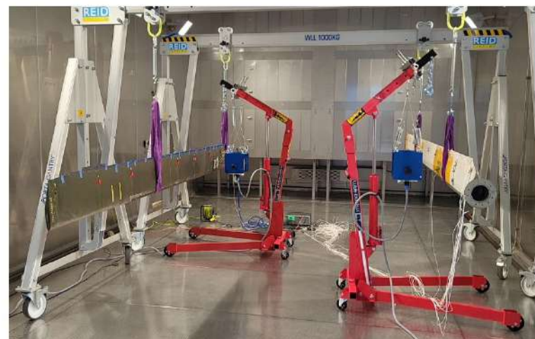
Figure 1. The experimental setup to perform modal testing on a metal (right) and composite (left) blade simultaneously.
